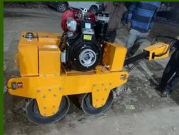
Vibratory Walk Behind 10HP Baby Roller Earth Compactor, 550 kg, Capacity: 2-3 Ton
